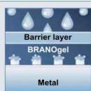
Volatile Corrosion Inhibitor (VCI): VCI forms a layer of protection on metal surfaces and displaces moisture. It repairs the passive layer and neutralizes the pH value. BRANOpac VCI formulations are considered most effective and the best in the world. VCI chemicals are specific for each metal. Please consult us for usage and storage guidelines.
