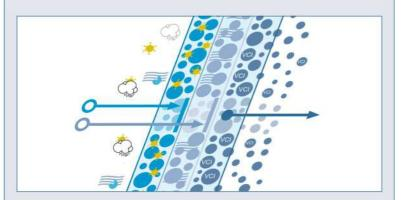
Firstly a perfectly harmonised system of high transparent barrier films provides a very low permeability of water vapor, oxygen and industrial air pollutant. On the other hand the established VCI system actively protects all types of metal components against corrosion in worldwide air, land and overseas transport.
