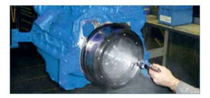
**BRANOtect** is a light corrosion protection fluid made from refined mineral oil, petroleum distillates and corrosion protection additives to ensure a highly effective protective film against corrosion. It contains neither silicones nor lanolin. It forms a highly effective temporary protective film against corrosion that has the ability to repair itself in the event of minor damage.
