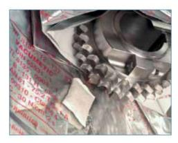
Vacumetic, Vacupac and Alfopac are aluminium composite films designed to meet application-specific usage situations. Together with BRANOgel they form an atmospheric packaging against moisture.
